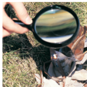
FIGURE 18–13 A converging lens can be used to start a fire in a pile of leaves.
