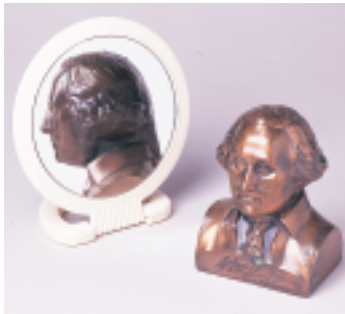
FIGURE 18-9 Objects placed between the focal point and the surface of a concave mirror form enlarged, virtual images.
