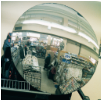
FIGURE 18–11 No real image is formed by a convex mirror. An erect, virtual image, reduced in size, is formed at the apparent intersection of the extended rays. Convex mirrors are often used as wide-angle mirrors for safety and security.
